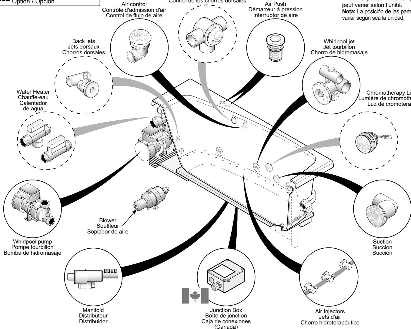
The whirlpool jets are individually adjustable. Using a finger, direct the jet nozzle inside the jet.
