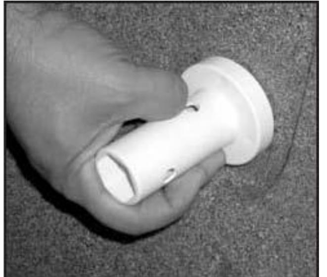
4. It is recommended to check and re-adjust the jet wall fitting using the short end of the jet wrench at least twice per year.
