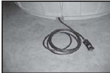
Pull G.F.C.I. along with power cord and inspect the full length of the cord for any damage before each use. If cord get's tangled, remove equipment access door. (see next picture)
