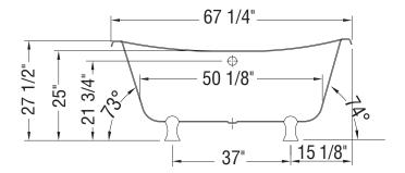
Bathtub base includes anti-vibration Neutra-Phone leg supports (not shown). All dimensions are approximate. Structure measurements must be verified against the unit to ensure proper fit.
