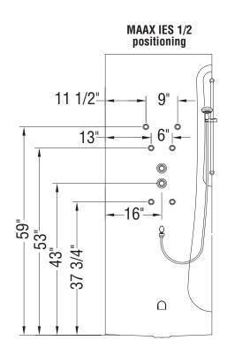
All dimensions are approximate. Structure measurements must be verified against the unit to ensure proper fit.
